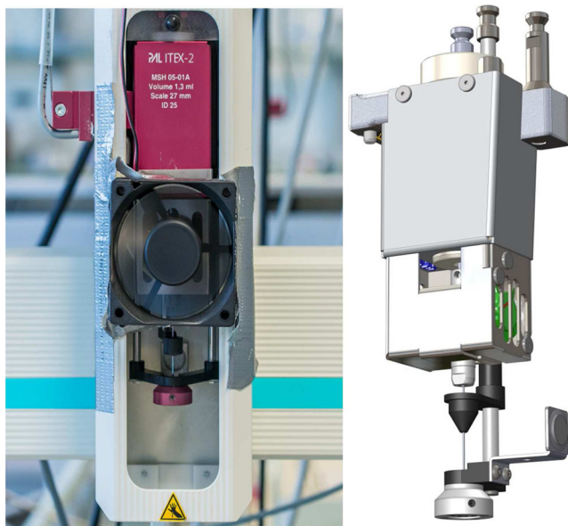
Fig. 9 Left Combi PAL modified with a 6-cm fan for trap cooling. Right ITEX DHS with implemented fan as it is distributed by CTC Analytik GmbH (Zwingen, Switzerland). Scheme with permission by CTC Analytik GmbH
