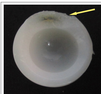
Figure 3 : Retrieved acetabular liner showing wear at the superior aspect (Solid arrow)
