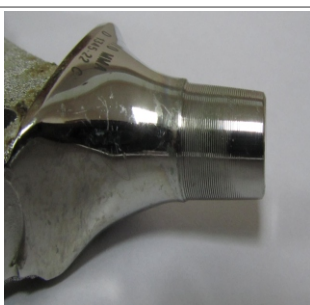
Figure 2 : Closeup of retrieved femoral component showing wear of the trunnion
