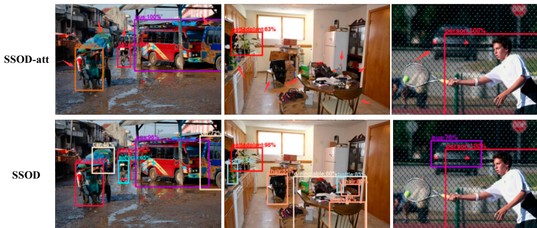
Figure 7. Comparison chart of detection effect between the SSOD algorithm and SSOD-att algorithm. The arrows indicate the objects detected by the SSOD algorithm but missed by the SSOD-att algorithm.
