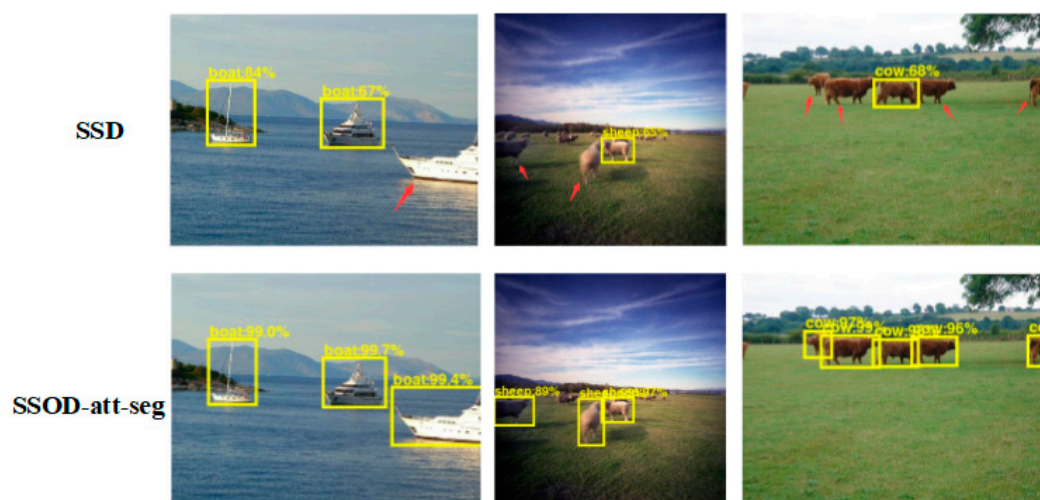
Figure 5. Comparison of detection effects between the SSOD-att-seg algorithm and SSD algorithm. The arrows indicate the objects detected by the SSOD-att-seg algorithm but missed by the SSD algorithm.
