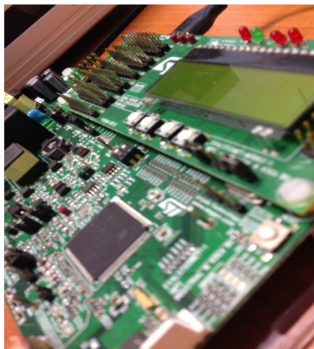
Figure 2. STMicroelectronics (ST) power-line communication (PLC) Evaluation smart meter board installed close-up with USB built-in debugging capabilities.
