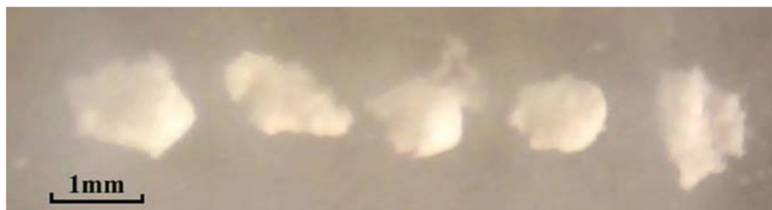
Figure 8. Dots of RespitoseSV003 monohydrate powder when the nozzle diameter is 500 \mu\text{m} .
