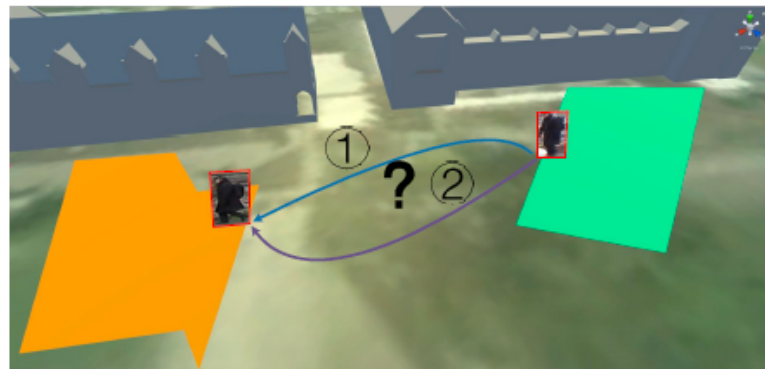
Figure 25. Event prediction in a blind zone [180]. This figure shows an example of two persons leaving the coverage of two different cameras (orange and green) and entering a blind zone. The video analytics system would predict and display the most probable trajectory of these individuals. The same concept could be used for the prediction of complex events such as criminal activity, possibly giving an operator extra time to respond.
