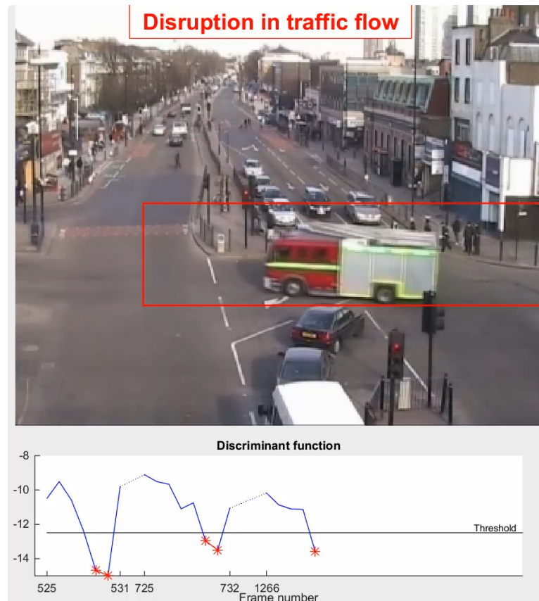
Figure 14. Multiple Object Detection with Topic Modelling [81]. The movement of the Fire engine, which is considered an abnormal event, in this case, is detected and marked with red boxes.
