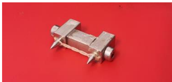
Fig 2. Designed holding-jig for retaining each of the chain segments
