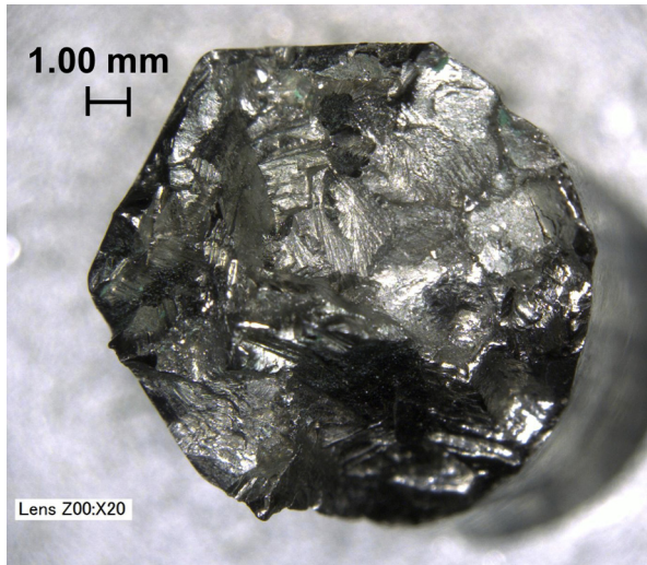
Figure 3. Low-magnification photographs reveal a large apparent grain structure at the location of fracture.
