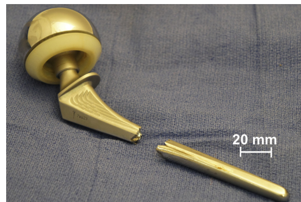
Figure 2. Photograph showing failure at the midportion of the stem, at approximately 38% of the stem length, measured from the collar.
