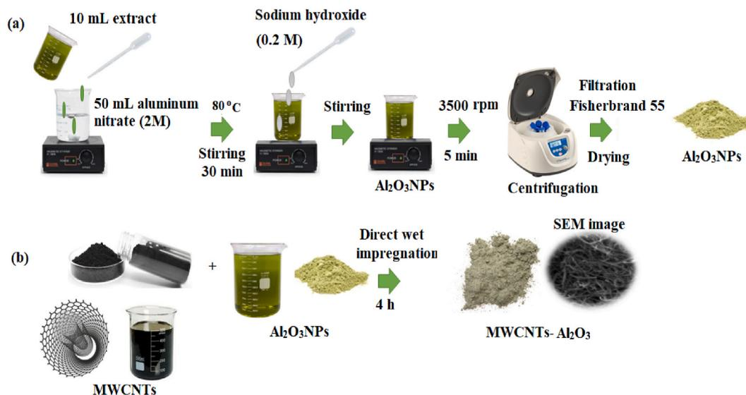
**Scheme 2.** (A) Preparation steps of Al<sub>2</sub>O<sub>3</sub>NPs and (b) functionalization of MWCNTs with Al<sub>2</sub>O<sub>3</sub>NPs using direct wet impregnation method.
