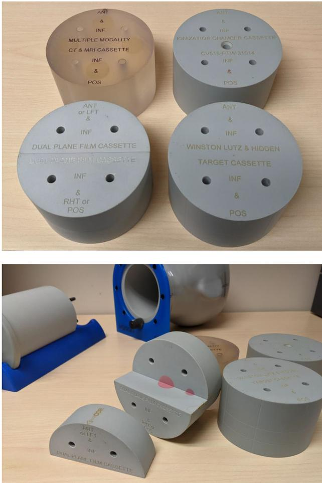
**FIGURE 2** Target cassettes used for dosimetric and geometric quality assurance. (Top) Four types of target cassette, clockwise starting upper left: multiple-modality computed tomography (CT) and magnetic resonance imaging (MRI), ionization chamber, Winston–Lutz/hidden target, and dual-plane film cassettes. (Bottom) One of the four segments that comprises the film cassette has been removed to show the contrast-enhanced (pink) targets used for planning
