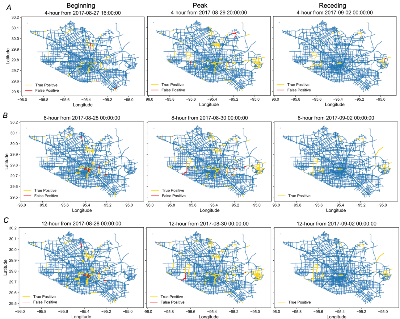
Figure 5. Examples of three prediction models for different phases of the flooding period (i.e., propagating, peak, and receding phases). (A) the model for predicting the situation in next 4 h; (B) the model for predicting the situation in next 8 h; and (C) the model for predicting the situation in next 12 h. The true positive (yellow) and false positive (red) road segments are all actual flooded road segments from the empirical INRIX data in a specific time interval.
