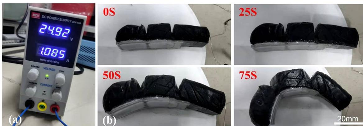
**Figure 6.** Electro-thermal driving test of the artificial finger. (a) DC power indicating the applied voltage and current for heating the artificial finger. (b) Captured photos recorded during the bending process of artificial finger in 75 s.
