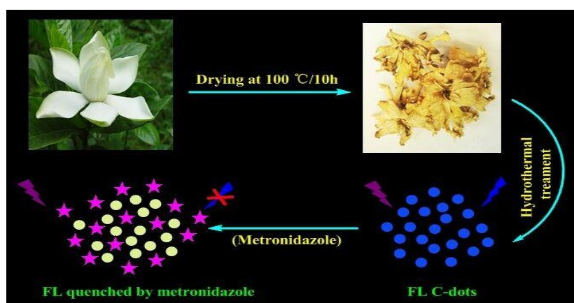
Scheme 1. Scheme of the synthetic strategy for FCNs and the principle of metronidazole sensing.
