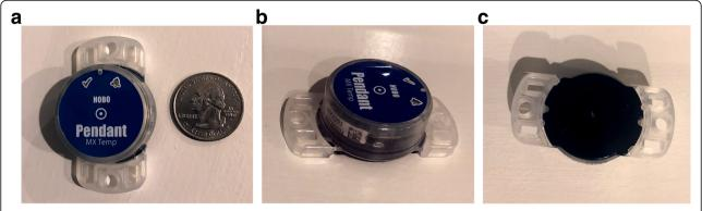
Fig. 1 Front (a), side (b), and back (c) views of the Onset Hobo MX2201 (Onset Computer Corporation, Bourne, MA)
