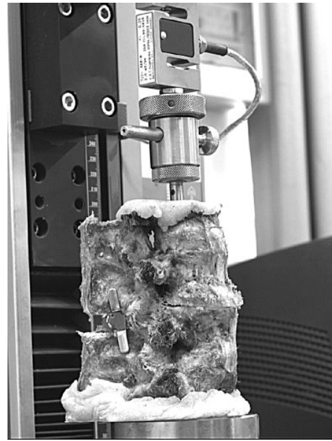
Fig. 2 The loading frame and the specimen being test
