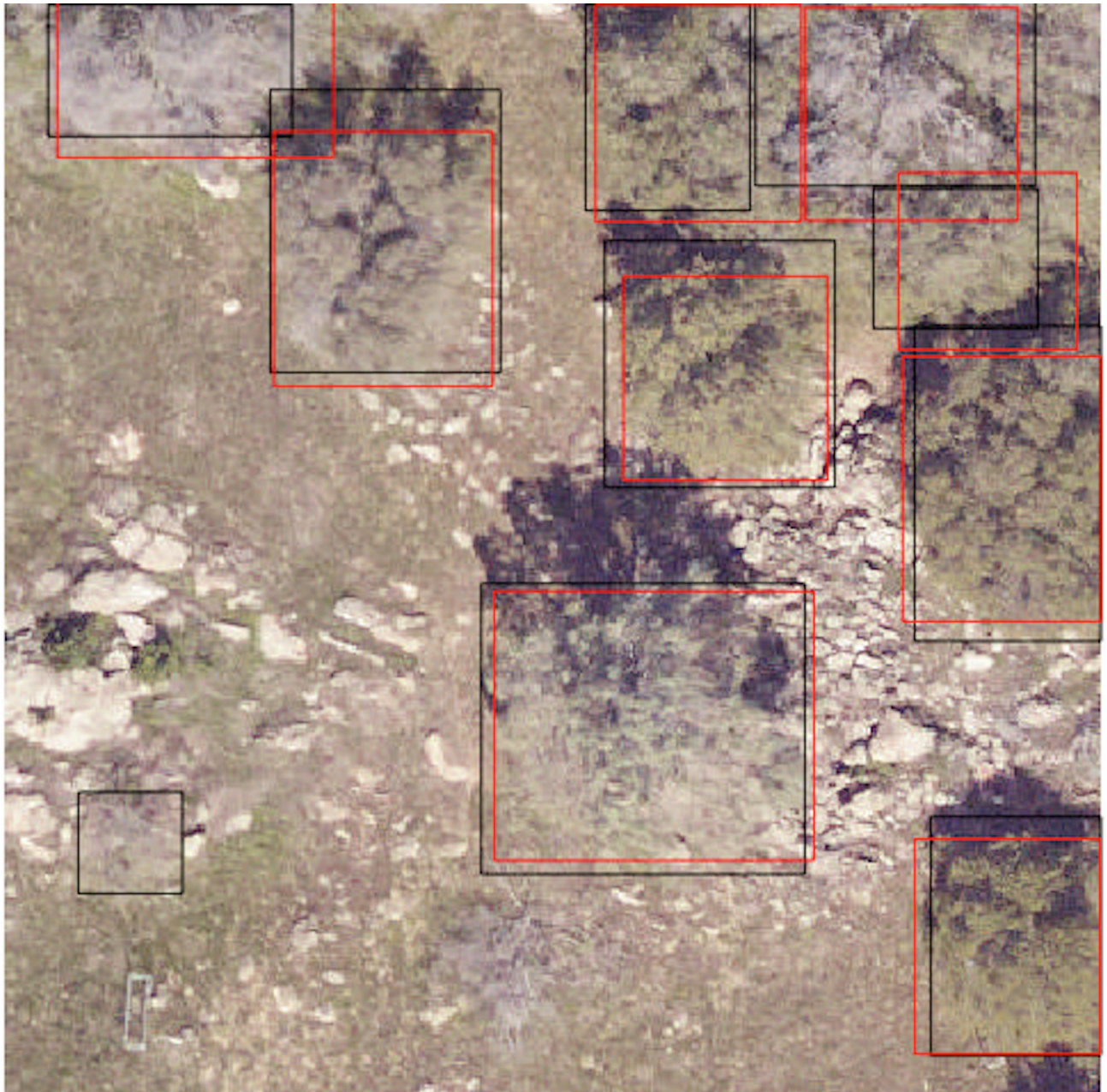
Fig 6. Example evaluation from the NeonTreeEvaluation R package. Predicted boxes (see below) in red and ground truth boxes are in black. In this image there are 10 image-annotated boxes, and 9 predictions. Each prediction matches an image-annotated box with an intersection-over-union score of greater than 0.4. This leads to a recall score of 0.9 and a precision score of 1.
