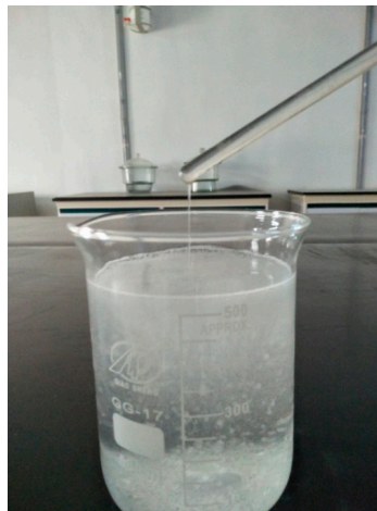
Figure 3. The appearance of the polyacrylamide (PAM) solution, which contains a large amount of suspended flocculates.
