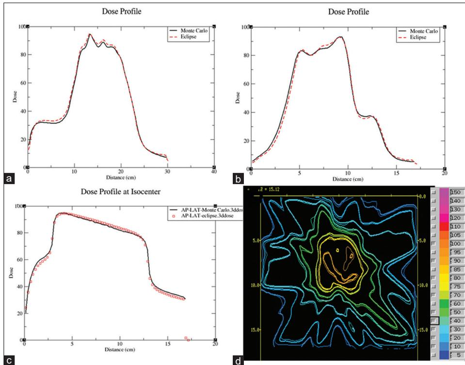
**Figure 1:** (a-c) show 1D comparisons of Monte Carlo and Eclipse AAA algorithm at the directions of anterior-posterior, superior-inferior and left-right respectively. (d) shows a 2D comparison of Monte Carlo (thin lines) and Eclipse AAA algorithm (thick lines)
