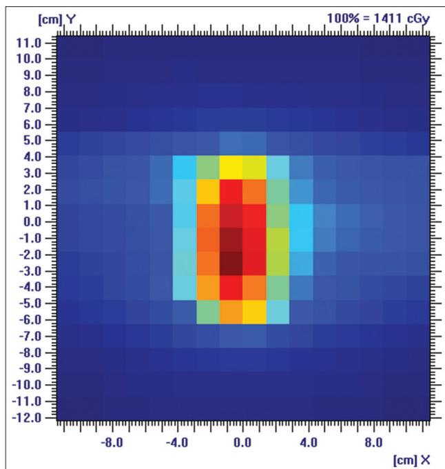
**Figure 4:** Ion chamber-based 2D measurements on case #2
