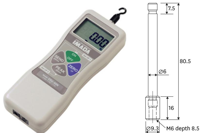
**Figure 1.** Digital force gauge (Model DS2-50 N, Imada, Tokyo, Japan) (left) and extension shaft (right), (unit=mm).
