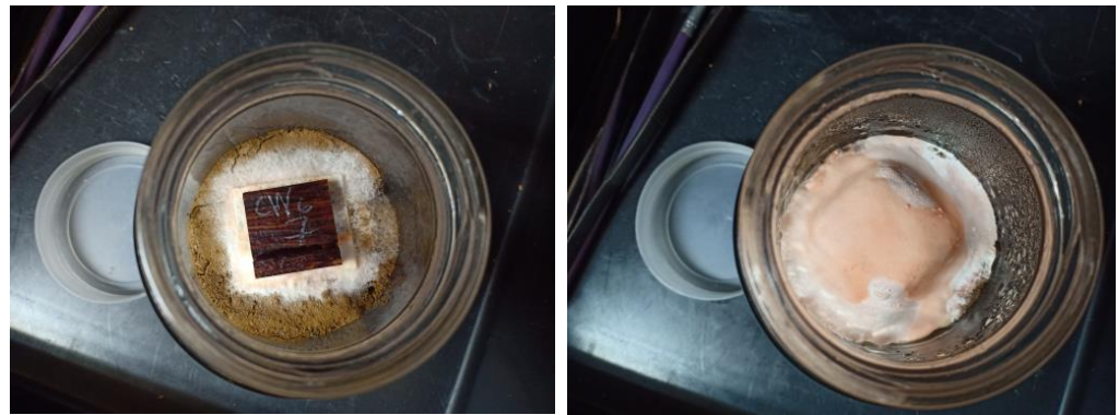
Figure 5. Fungal growth observation of the MGE plywood (left) and control (right) after 8-week exposure to white rot fungi.
