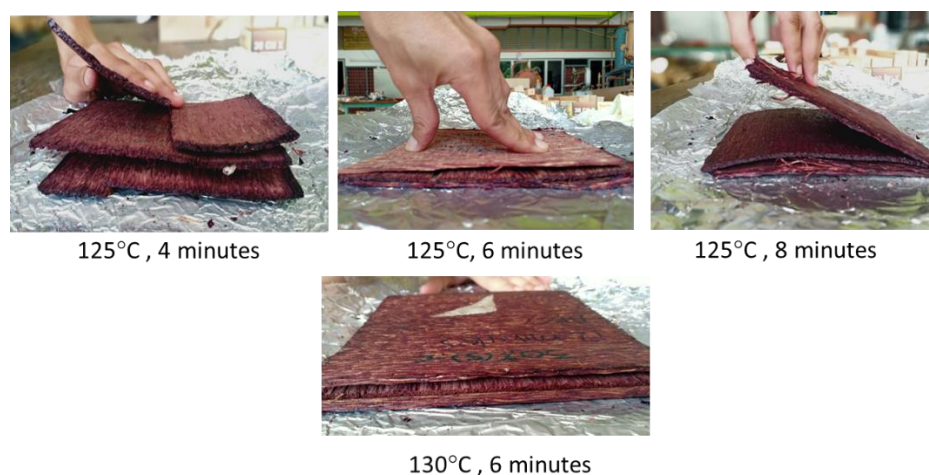
Figure 3. Plywood produced using designated pressing temperatures and times showed failure in bonding.
