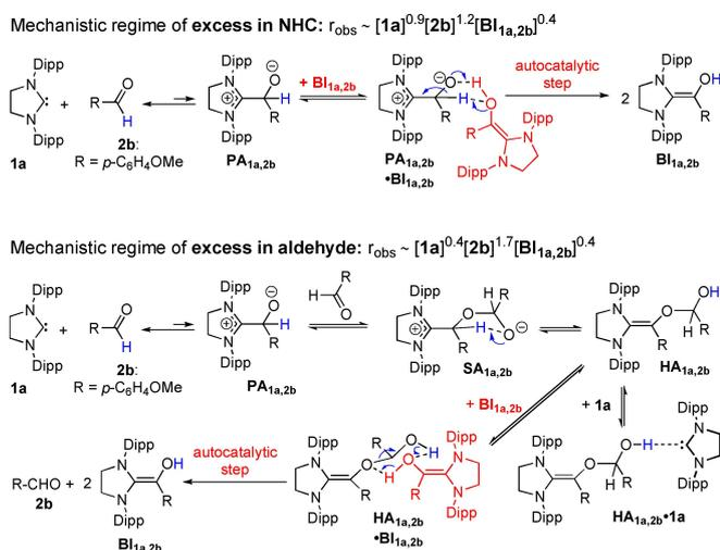
**Scheme 4.** Mechanistic proposal for the reaction of SIPr (**1a**) with anisaldehyde (**2b**) to the Breslow intermediate **BI**<sub>1a,2b</sub> under aprotic conditions. Top: in the presence of excess SIPr (**1a**); bottom: in the presence of excess aldehyde (**2b**).
