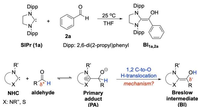
**Scheme 1.** Formation of Breslow intermediates (BIs) from N-heterocyclic carbenes (NHCs) and aldehydes under aprotic conditions; top: reaction of SIPr (**1a**) with benzaldehyde (**2a**); bottom: the crucial 1,2-C-to-O proton shift in the conversion of the zwitterionic primary adduct (PA) to the Breslow intermediate (BI).
