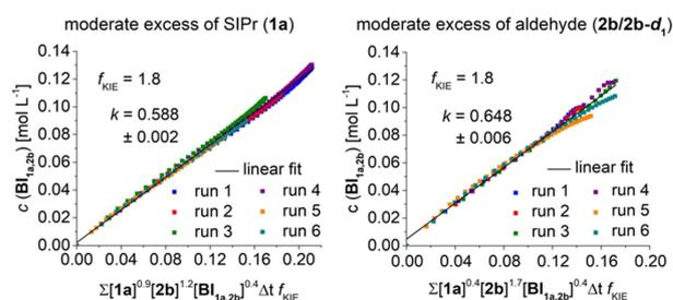
**Figure 3.** Variable time normalization analysis (VTNA), with additional normalization factor  $f_{KIE}$ ; left: moderate excess of SIPr (**1a**), compare with Figure 1; right: moderate excess of anisaldehyde (**2b**), compare with Figure 2. In both cases,  $f_{KIE}=1.8$  gave best overlap and linearity ( $R^2=0.99$ ).
