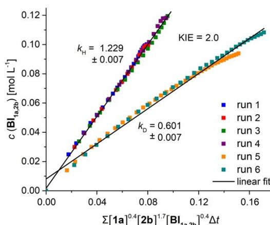
**Figure 2.** Variable time normalization analysis (VTNA), excess of anisaldehyde (**2b**): reaction order of 0.4 in SIPr (**1a**), 1.7 in anisaldehyde (**2b**) or anisaldehyde-*d*<sub>1</sub> (**2b-d**<sub>1</sub>), and 0.4 in Breslow intermediate **BI**<sub>1a,2b</sub> gave best overlap ( $R^2=0.99$ ). Concentration-time profiles of the reaction of **1a** with **2b** or **2b-d**<sub>1</sub> were obtained by <sup>1</sup>H NMR, (400 MHz, THF-*d*<sub>6</sub>, 298 K).
