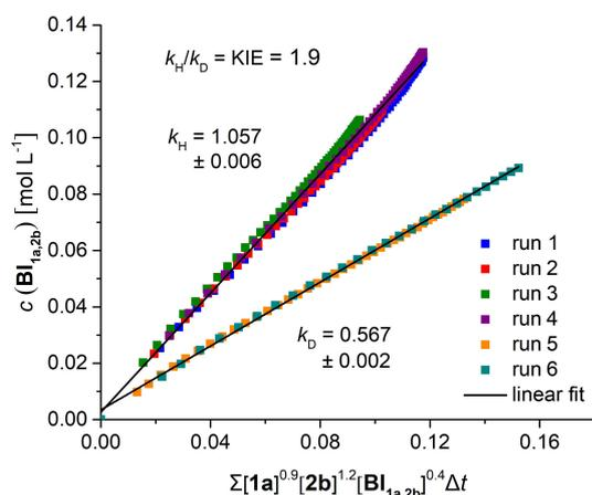
**Figure 1.** Variable time normalization analysis (VTNA), excess of SIPr (**1a**): reaction order of 0.9 in SIPr (**1a**), 1.2 in anisaldehyde (**2b**) or anisaldehyde-*d*<sub>1</sub> (**2b-d**<sub>1</sub>), and 0.4 in Breslow intermediate **BI**<sub>1a,2b</sub> gave best overlap ( $R^2=0.99$ ). Concentration-time profiles of the reaction of **1a** with **2b** or **2b-d**<sub>1</sub> were obtained by <sup>1</sup>H NMR, (400 MHz, THF-*d*<sub>6</sub>, 298 K).
