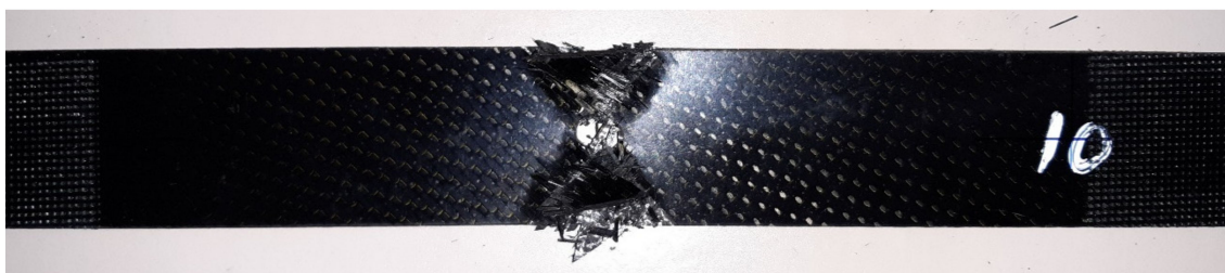
Figure 17. AIR-3R failed specimen under OHT test.
