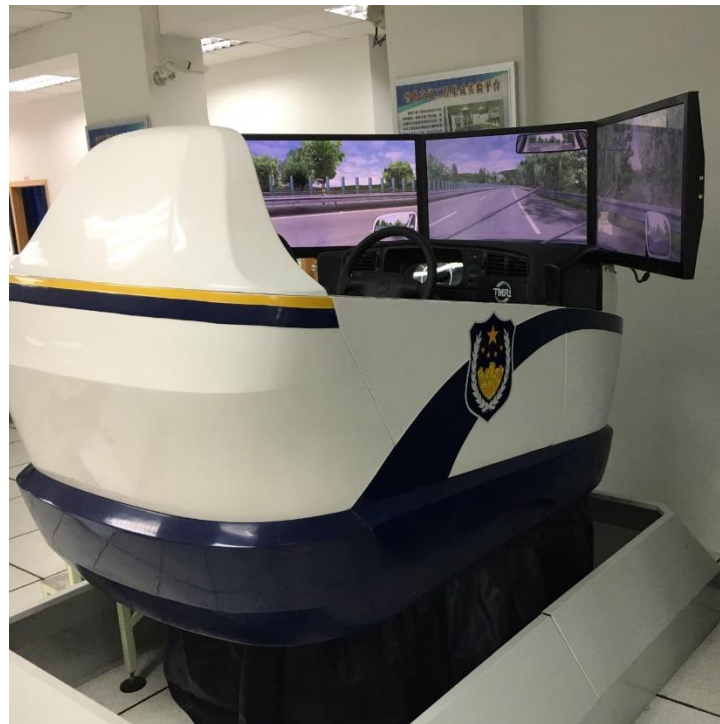
Figure 1. Fix-based driving simulator in the South China University of Technology.
