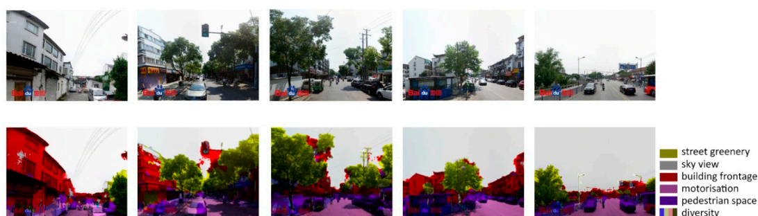
Figure 7. Applying SegNet to extract key spatial elements.
