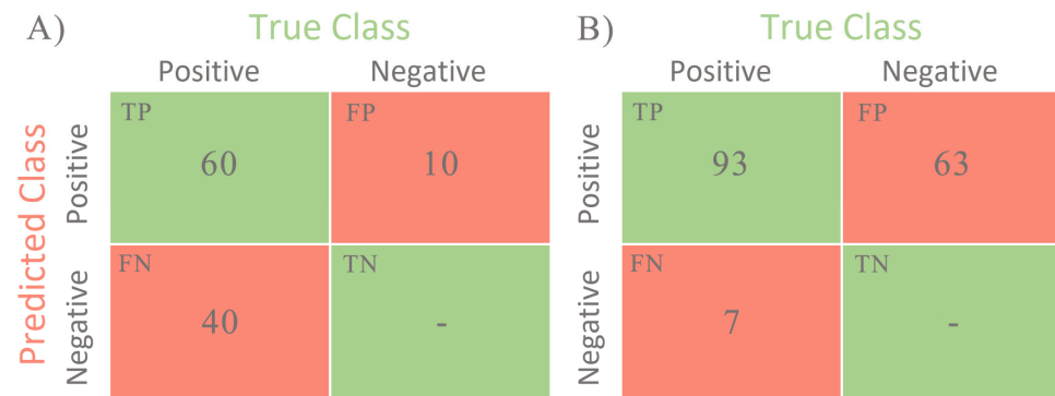
Figure 10. Confusion matrixes for (A): YOLOv4-based method and (B): NCA-based method. TP—the model detected a lesion where it actually exists; FP—the model detected a lesion where it actually does not exist; FN—the model did not detect the lesion, where it actually exists.
