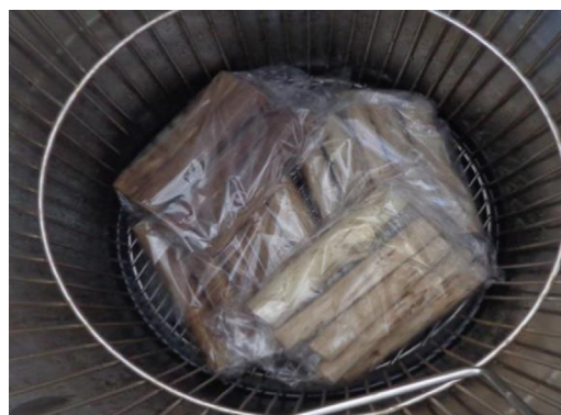
Fig. 1. Sterilization of debarked poplar billets inside polypropylene bags.
