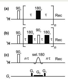
Fig. 1 Pulse sequences for measuring  $T_2$  relaxation: (a) CPMG, (b) PROJECT, and (c) TRUE using a Zangger-Sterk (ZS) element. The decay of the NMR signal is measured as a function of n in each case.
