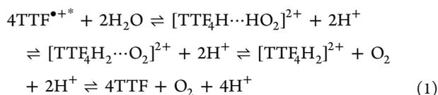
Electrochemical recycling of TTF<sup>•+</sup> on GF:
