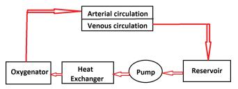
**Figure 1:** During CPB, venous blood is drained through gravity into a reservoir. The pump moves blood from the reservoir to the oxygenator through a heat exchanger, before returning it to the arterial circulation. Additional components include suckers (to remove blood from surgical field), vents (to decompress the heart), haemofilters (for ultrafiltration) and cardioplegia system
