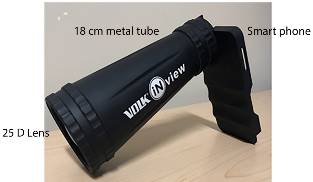
Figure 2. Housing and optical principles of smartphone retinal imager. The 25D condensing lens sits approximately 4.8 cm from the eye at the farthest end of the 18 cm metal tube, which is attached to the smartphone. The smartphone-based fundus camera allows for creation of an inverted, real aerial image approximately 6.6 cm from the condensing lens.
