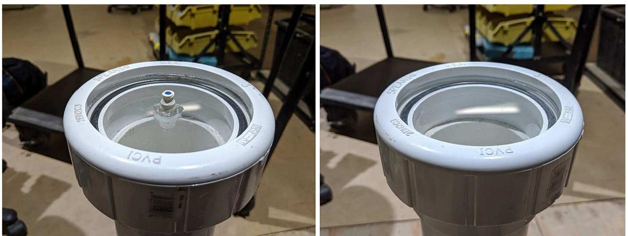
**Fig. 6.** PAWS housing with PVC union threaded endcaps and collars. The front and rear doors (left and right respectively) are made from laser cut clear acrylic. The pass through in the front door is an IV valve epoxied into a laser cut, or drilled, hole through the center of the disc.
