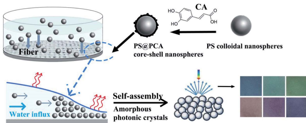
Fig. 1 Preparation of biomimetic non-iridescent structural color based on polystyrene–polycaffeic acid core–shell nanospheres.
