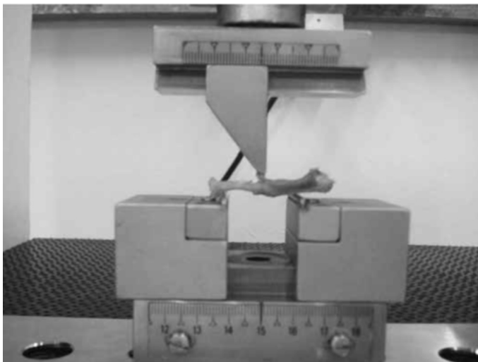
Figure 3 – Fractured tibia undergoing three-point mechanical flexion test. Source: University of Uberaba.
