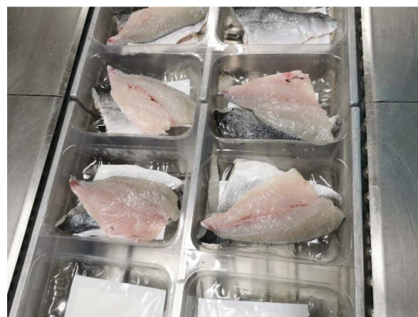
Figure 1. Packaging of gilthead seabream fillets in a thermoforming machine for modified atmosphere packaging with a CO 2 emitter pad.
