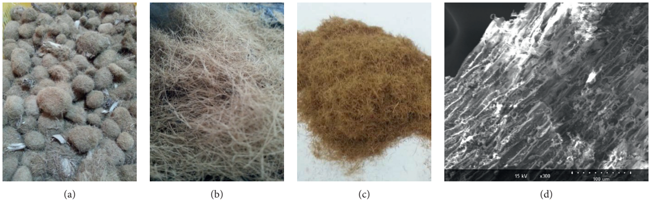
FIGURE 1: Posidonia oceanica (PO) used as biosorbent: (a) collected balls, (b) separated raw fibers, (c) milled and sieved PO fibers, and (d) SEM of PO fibers.
