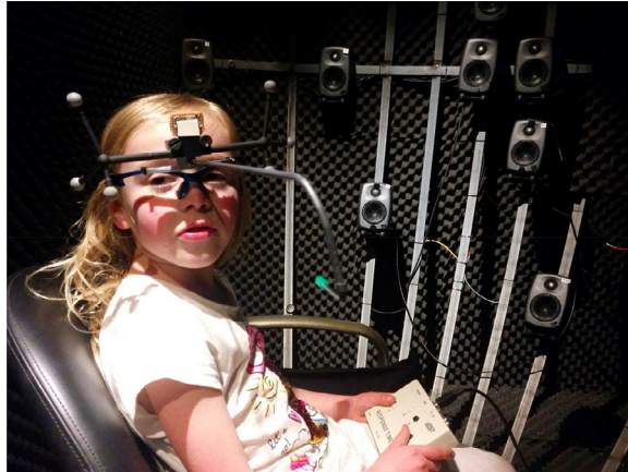
Fig. 3. Frame with 3 infrared reflectors mounted on both sides and a green LED on a pointer centrally fixated in front of the participant's nose.
