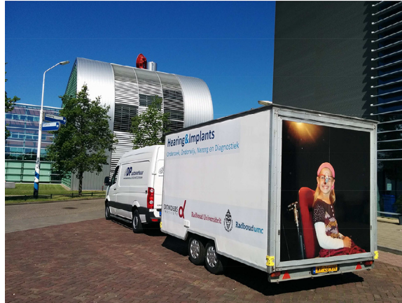
Fig. 1. Mobile localization lab in a sound-isolated anechoic trailer.
