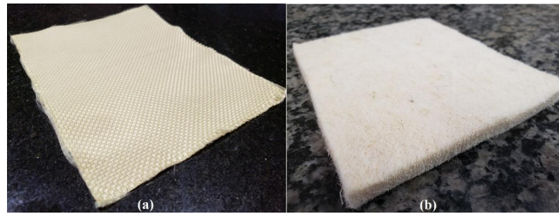
Figure 2. (a) Aramid woven fabric and (b) curaua non-woven mat.
