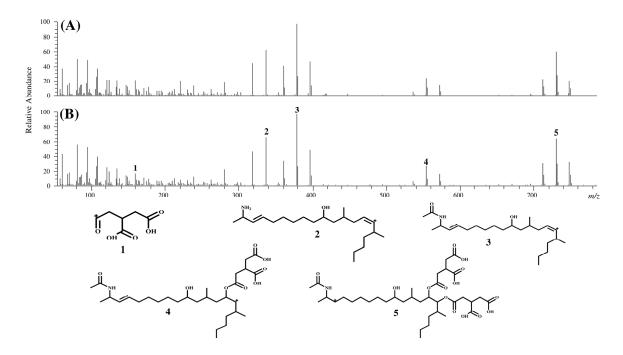
**Figure 4.** Product ion spectra of compound III and FA3, and characteristic peak assignment of FA3. (A) Product ion spectrum of compound III; (B) product ion spectrum of FA3.
