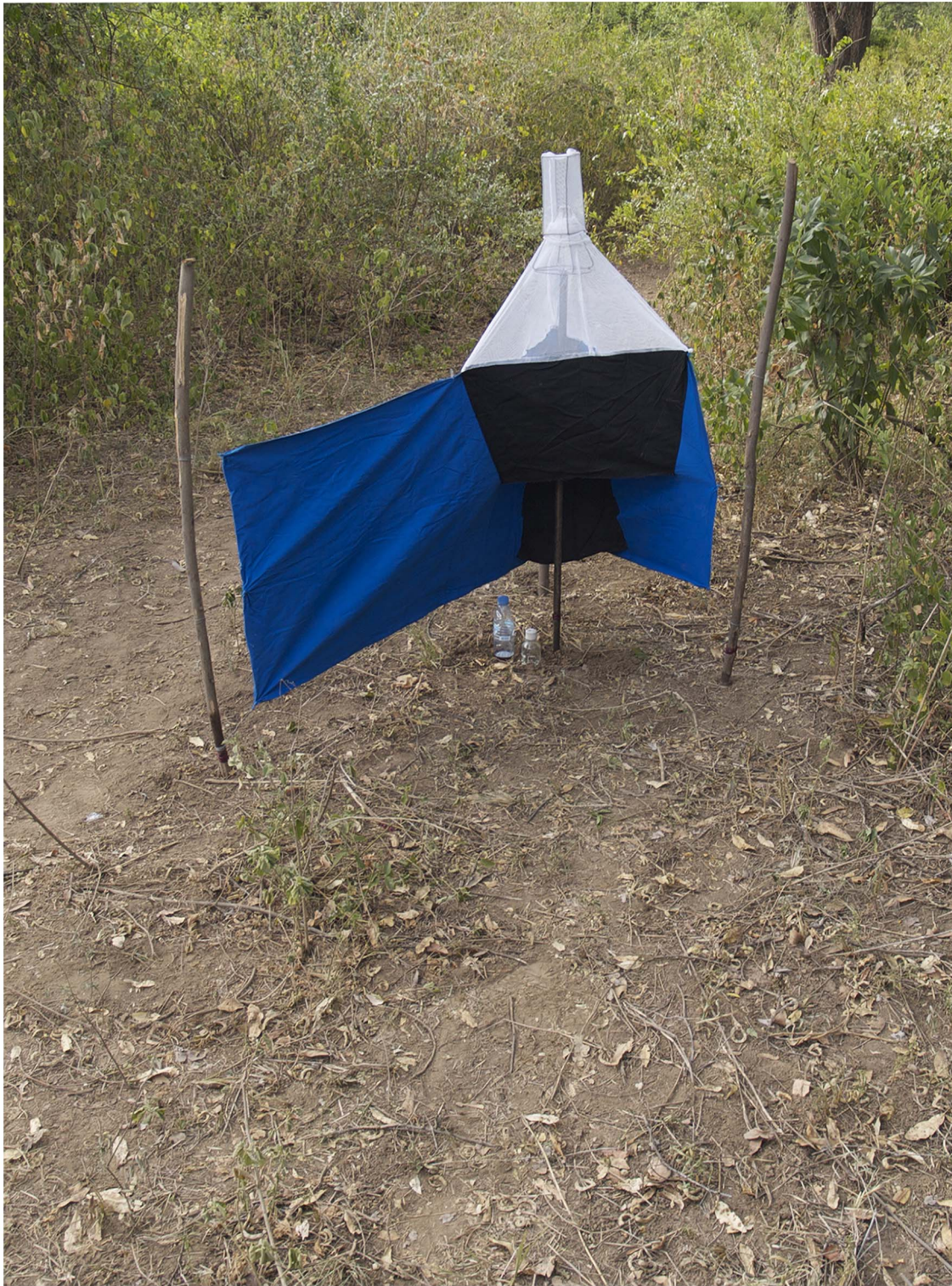
Figure 2. A Ngu trap (named after Nguruman, where it was developed) developed for savannah species of tsetse flies. The baited trap is based on both visual (shape and colour) and olfactory cues (e.g., using cow urine and acetone). doi:10.1371/journal.pntd.0002687.g002
