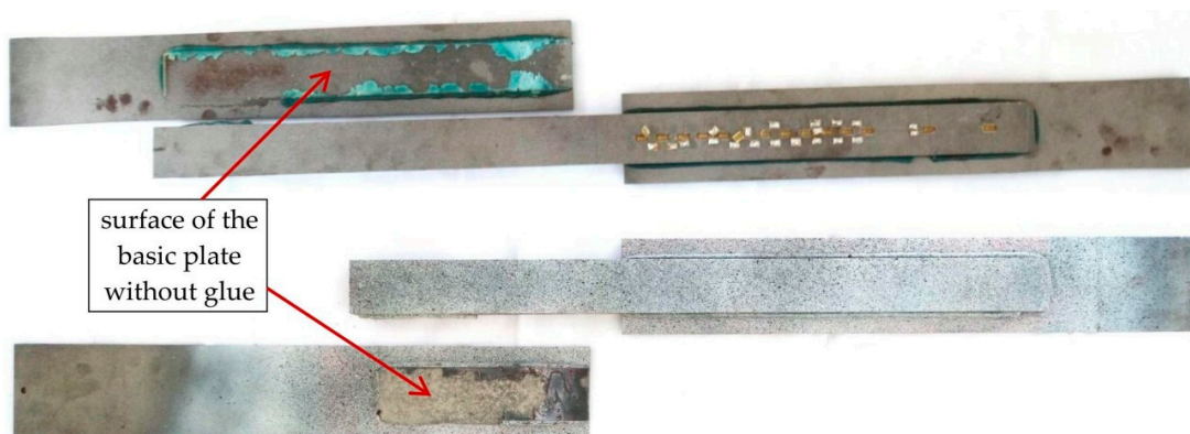
Figure 8. The specimens after failure: Above the element from series S/DL/MA/RS-400/P1 and below the element from series S/DL/MA/RS-200-4/P2.
