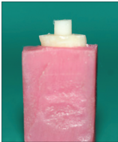
Figure 3: Specimen with glass ionomer cement after the removal of polyvinyl mold
