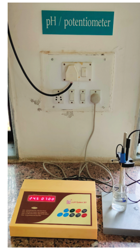
Fig. 2: Digital pH meter used for adjusting the PH of remineralizing solution at 7.0
