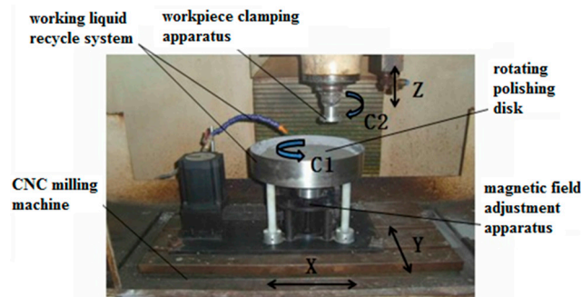
Figure 2. Experimental apparatus for cluster MR effect in plane polishing.
