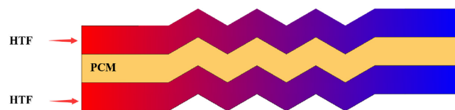
Figure 12. Sawtooth plate heat storage structure.
