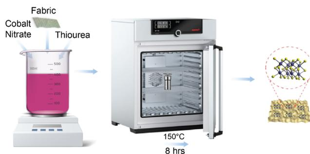
**Figure 1.** Synthesis of  $Co_9S_8$  using the hydrothermal method.
