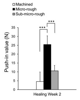
**Figure 5.** The strength of implant anchorage in bone, evaluated by the biomechanical push-in test in a rat femur model. Each bar represents mean  $\pm$  standard deviation of machined (n = 5), micro-rough (n = 5), or sub-micro-rough (n = 5) titanium. \*\*\* p < 0.001, one-way ANOVA followed by Tukey's test.
