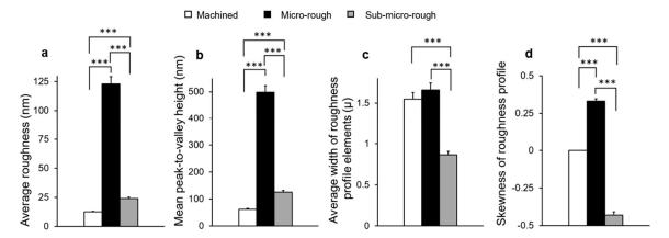
**Figure 2.** Quantitative measurements of surface roughness of the machined, micro-rough, and sub-micro-rough surfaces using a 3-dimensional profiler. (a) Average roughness, (b) mean peak-to-valley height, (c) average width of roughness profile elements, and (d) skewness of roughness profile. Each value represents the mean  $\pm$  standard deviation of six sites on the three different surfaces (n = 6). \*\*\* p < 0.001, one-way ANOVA followed by Tukey's test.
