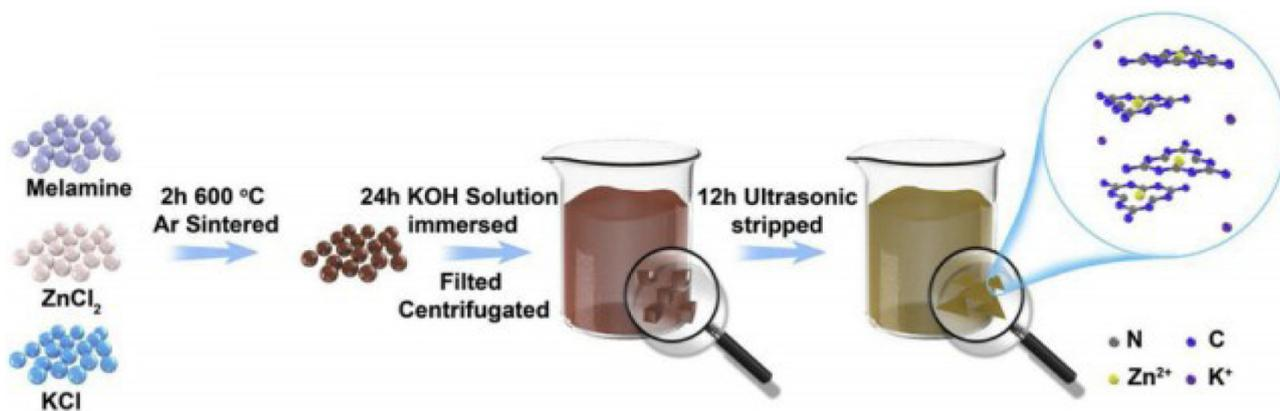
**Fig. 9. – Schematic of the preparation for  $\text{Zn}^{2+}, \text{K}^+ - \text{C}_3\text{N}_4$  nanosheets. Reproduced with permission from [33]. Copyrights 2020 Elsevier B.V.**
