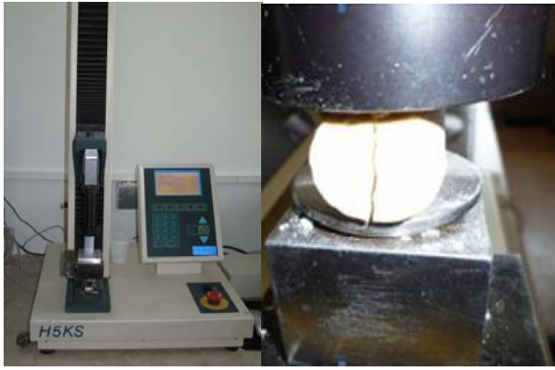
Figure 2. Mechanical testing machine (A). Measuring the tensile strength of the stone model (B).
