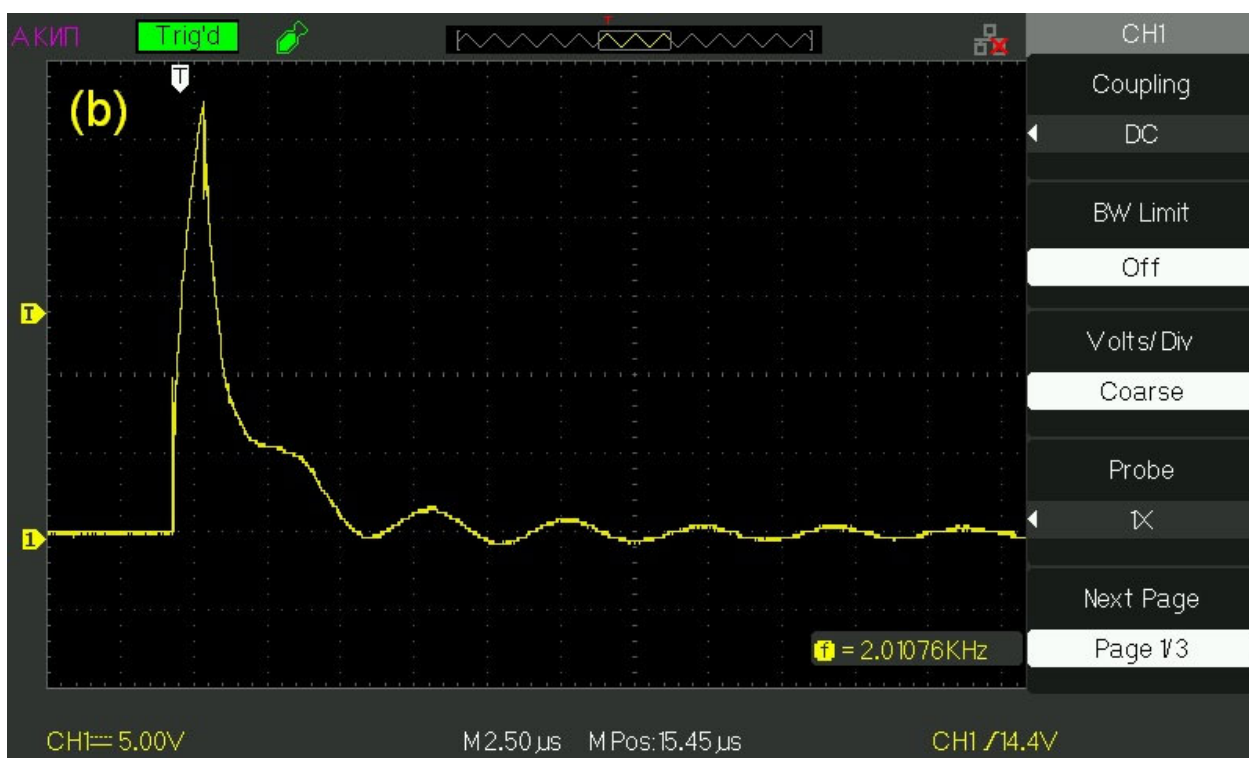
Figure 2. The oscillograms of electrical pulses that were fed to a piezoelectric transducer. Panel (a)—the transducer is not immersed in water. Panel (b)—the transducer is immersed in water.
