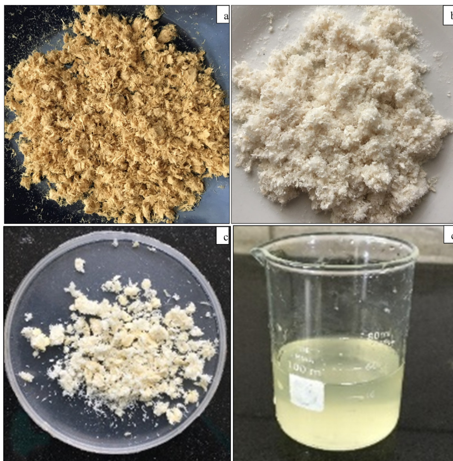
Figure 5. a) Unbleached pulp; b) bleached pulp; c) dried nitrocellulose; d) nitrocellulose lacquer.
